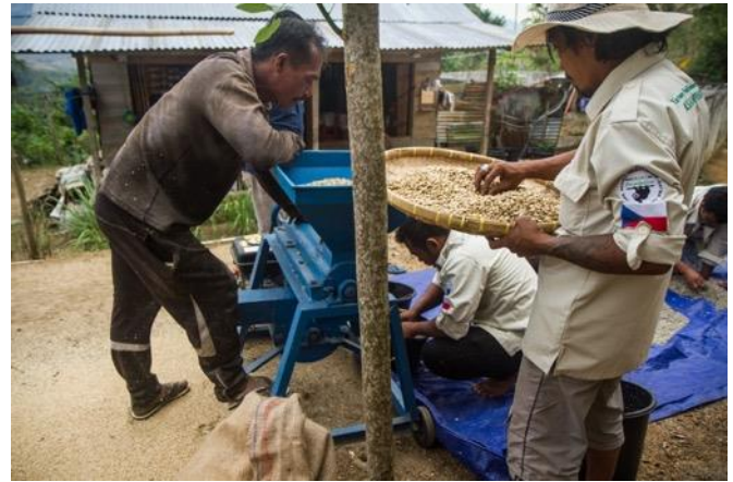
Peeling of parchment with a new peeler
